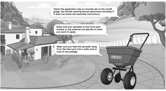
Check the material to be applied is dry and free flowing to ensure it will flow freely through the hopper. Make sure your application rate and spread pattern settings are correct, **close the application hole fully** and then pour in your material.
