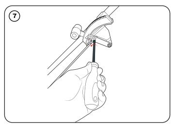
Tighten the control rod.
