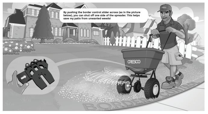
To protect your borders simply slide the border control into position to cut off the left hand side of the spread pattern.
