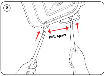
Align the holes at the bottom of the handle bar(item 2) with the holes at the top of the lowerframe (item 14). You may need to pull the endsapart slightly to place in position.
